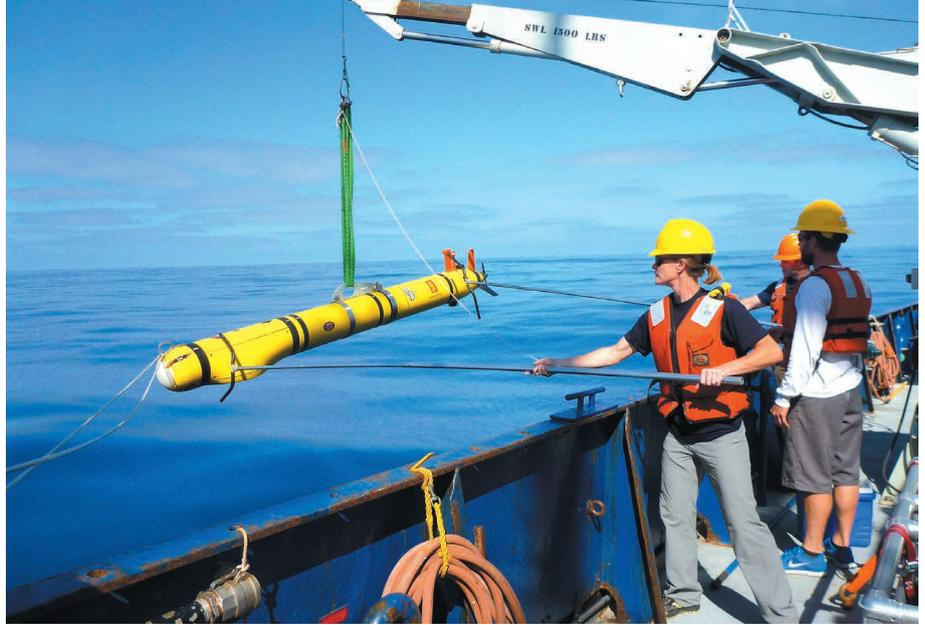
This customized autonomous underwater vehicle has sonar devices to detect marine animals.
